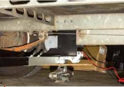
**3.** Fit and secure the motor assemblies, keeping the mounting bolts finger tight. Using some duct or gaffer tape, take the supplied spacer and secure it to the unengaged drive rollers. These need to be positioned 20mm from the tyre on the caravan. This precise distance is critical to the operation of the unit.
