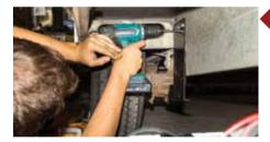
2. Position the adaptor plates on the chassis, and clamp the plates in position as per the instructions. Mark the spots to drill, tap with a centre punch then drill three holes through the chassis rails. Fit the supplied nuts and bolts and finger-tighten.
