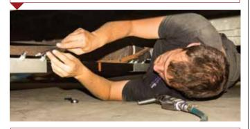
**6.** Slide the motor and drive rollers towards the van's tyre until it sits tight up against the spacer. Once everything has been positioned correctly, tighten all bolts to 40lb.ft using a torque wrench, except the crossbar pinch bolt/lock nut. The crossbar doesn't need to be tightened as much, and only requires 9lb.ft of torque to comply with the manufacturer's specifications.
