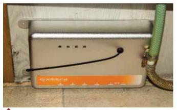
**7.** Mount the supplied electronic control unit (ECU) in a secure position using the four screws that are supplied. Spend some time thinking about where to mount the ECU, as it needs to be away from dust and water, and still close enough to the battery to keep wiring to a minimum.
