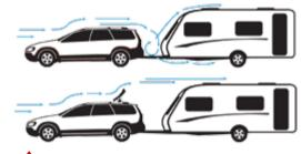
Aeroplus deflects wind right over the top of your van, reducing wind turbulence and resistance
