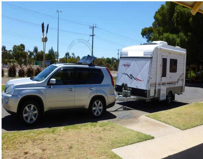
consumption was **13.4 litres per 100km**. This is an improvement of over **20%**. Wind direction was averaged out to be almost the same. From Penong to Norseman the car is mostly climbing from 50m, up to 420m. So on the return trip the car is dealing with higher temperatures and a climb, plus the additional accumulated weight. Averaged out, for the overall trip, you would more than likely return a **15% fuel saving**.
