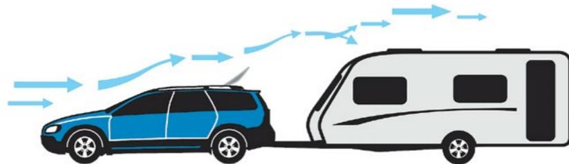
Roof-mounted air deflector that drives the flow of air smoothly over the top of your caravan.
