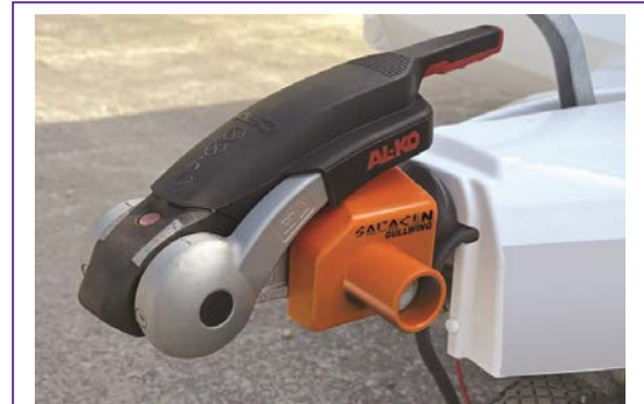
Purple Line's new Saracen Gullwing provides security for vans fitted with European-style AL-KO hitches.
